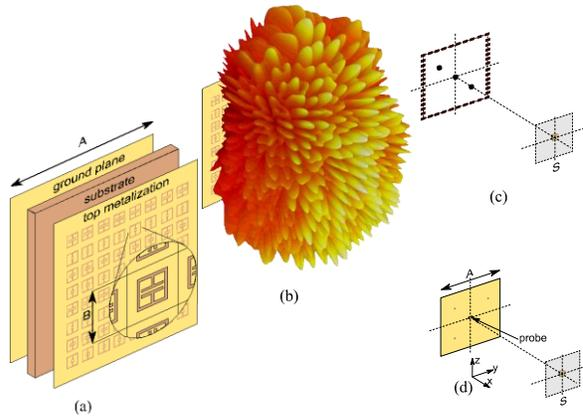
FIGURE 1(a) An illustration of the metamaterial parallel plate antenna with characteristic cELC resonators etched into the top layer. (b) A plot of the radiation pattern of the metamaterial panels at a fixed frequency is shown. (c) The SAR imaging configuration used in the PSF analysis is shown, with a single voxel as a target in the region of interest S; (d) The modeled one panel and one probe frequency diverse imaging system is illustrated.
